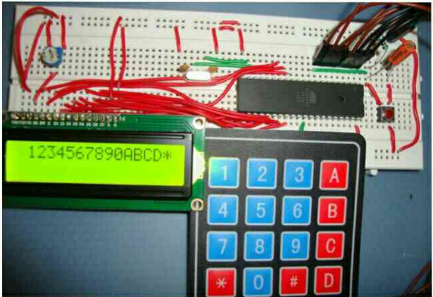
4x4 Matrix Keypad Interfacing with 8051 Microcontroller
