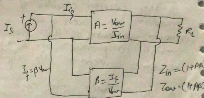
Voltage feedback tends to reduce the output impedance
