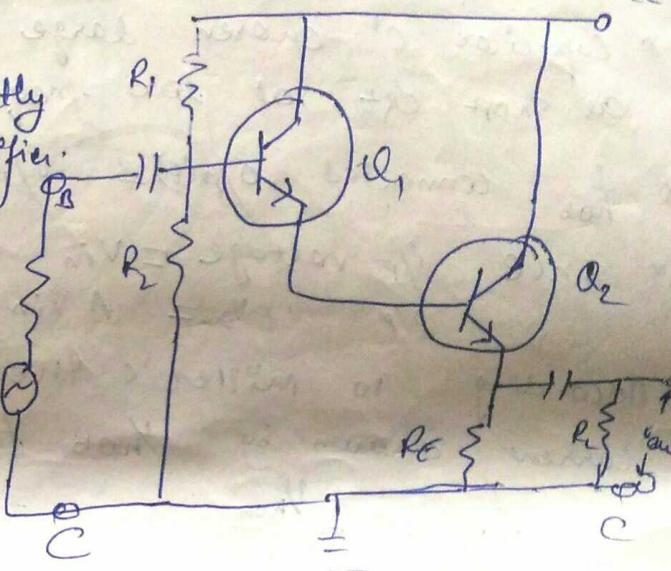
I/P impedance  $\rightarrow$  of the darlington Amplifier is higher than a single amplifier.
