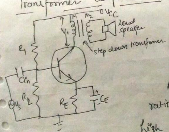
Transformer for coupling the load to the amplifier is usually employed.
