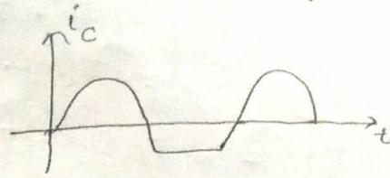
Class C :- operates for less than  $180^\circ$
