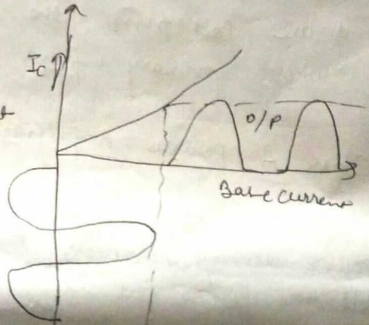
Harmonic distortion: - Caused due to non-linearity of the active device employed for amplification.
