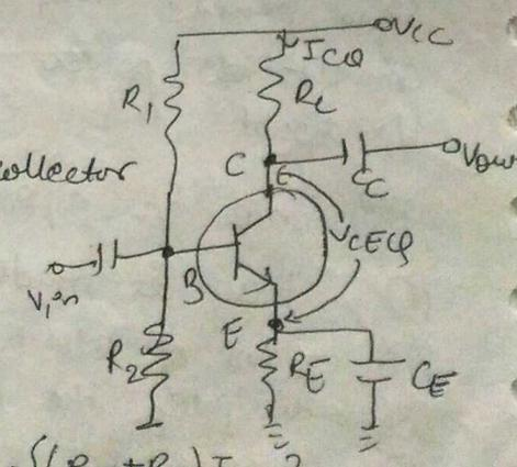
be eliminated because it is a part of biasing n/w &  $R_C$  can't be short ckt if  $R_C$  is short circuited  $R_E$  will be short-circuited and there will be no transfer of power to the  $R_L$ .
