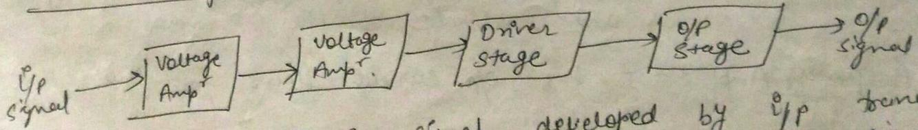
(A) Voltage Amplification :- signal developed by i/p transducer is very small and need amplification. so for raising level of weak signal, it is amplified in two or more stages.
