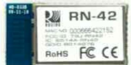
This address should be visible on most Bluetooth devices. For example, on this RN-42 Bluetooth Module, the address printed next to "MAC NO." is 000666422152. The "000666" portion of that address is the OUI of Roving Networks, the manufacturer of the module. Every RN module will share those upper 24-bits. The "422152" portion of the module is the more unique ID of the device.
