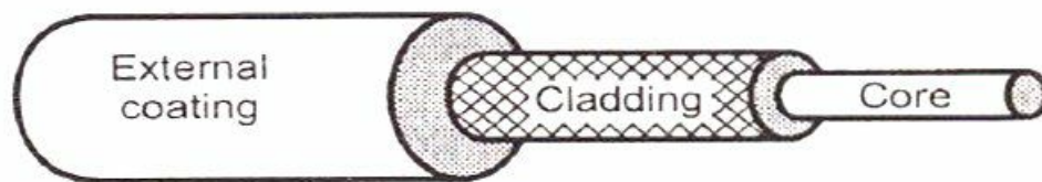
Fig. 1.6.6 Single optical fiber structure
